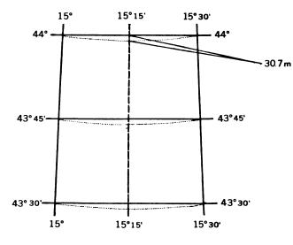
The 15',  $x = 15'_{\lambda}$  sheets at 1:50,000 scale should be independently constructed as isosceles trapezoids then the rise between the 15' arc of parallel and respective chord at the center of Yugoslavia
