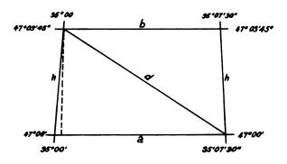
The sheet lines were computed by formulae used in the computation of basic graticule sheet  $15'_{0} \times 30'_{1}$  (See page 30)
