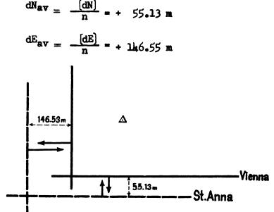
According to the preface of "Positions Rechnungen" (Protocol 290 A) the plotted positions in this area were adjusted along with the conversion of geographic positions into rectangular coordinates. In order to avoid the creation of the overlapping strips along the junction of the sheets of the two systems, the empirically adjusted positions were plotted on plane table sections and the sheets of both systems were matched by a gradual shift of the sheet lines.
