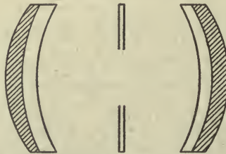
*FIG. 64—DOUBLE COMBINATION LENS
