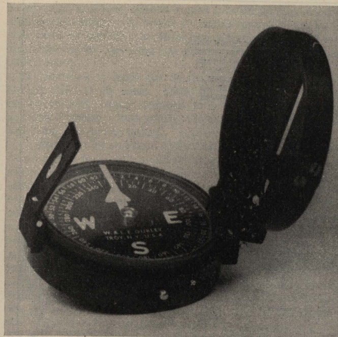
② FIGURE 51.—Lensatic compass—Continued.
