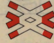
DOUBLE TRACK LEVEL CROSSING NO GATES
